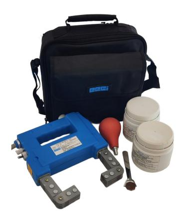
The EECIFLUX MPI Kranti Kit is a comprehensive solution for magnetic particle inspection (MPI) applications, designed for efficiency and reliability. This kit includes all the necessary components for conducting dry application with yoke MPI inspections with ease, making it ideal for new users, training institutes, and industries.
